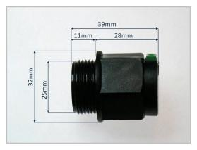
Recommended panel cut-out : Ø 25 mm Max panel thickness : 6 mm Weight 30 gram
